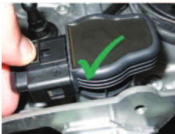
Figure 1. Correct method of disconnecting the ignition coil.
