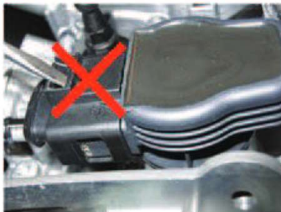
Figure 3. Incorrect method of disconnecting the ignition coil.
