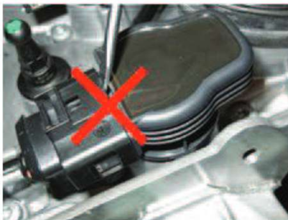
Figure 2. Incorrect method of disconnecting the ignition coil.
