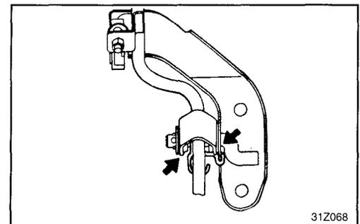
2. To prevent entry of exhaust fumes, apply semi-drying type sealant to the bolt mounting hole, and then tighten the accelerator arm bracket.
